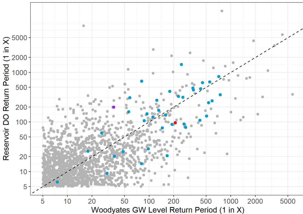
Figure 2-34 Stochastic drought events plotted against reservoir and Woodyates groundwater level return period, alongside selected stochastic drought library events (blue), 1975/76 historical drought (red) and 1921 historical drought (purple)
