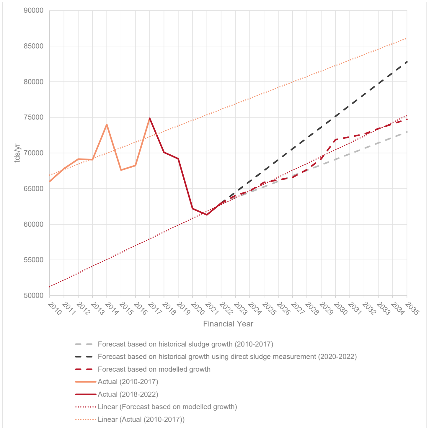
Figure 25 – Forecast sludge production using modelled sludge production growth rate and historical sludge production growth rates in Table 18
