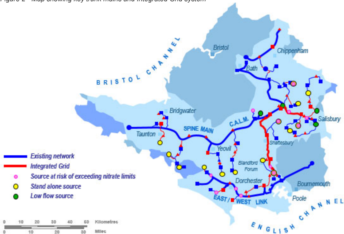
Figure 2 - Map showing key trunk mains and Integrated Grid system
