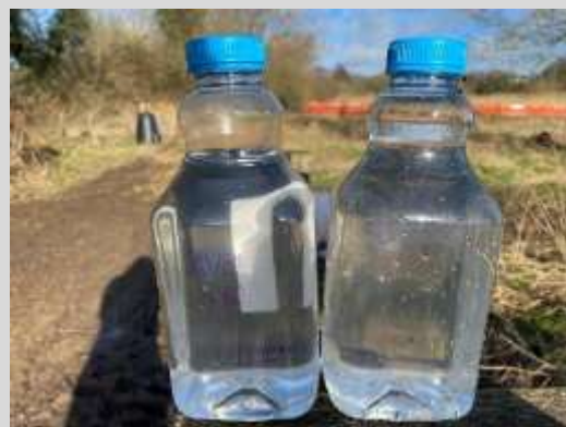
River water quality (left bottle) and influent to reed-bed (right bottle) showing the clarity of the ‘raw sewage’ that passes through the natural treatment process.
