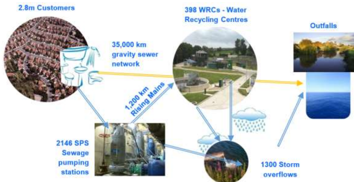
Figure 9: Wessex Water wastewater asset statistics
