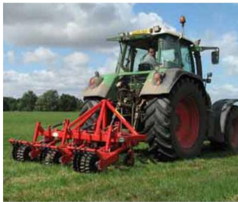
A grassland subsoiler / swardlifter at work and it's key components. Photo credit: Adas
