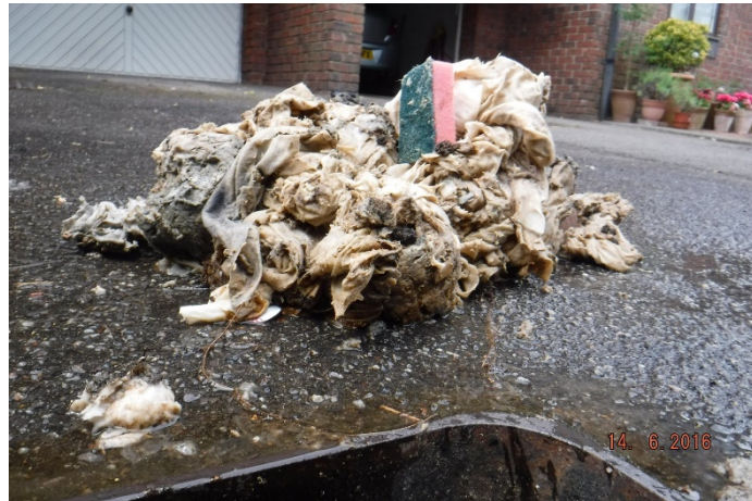
Figure 15: Typical example of wet wipes removed from a sewer
